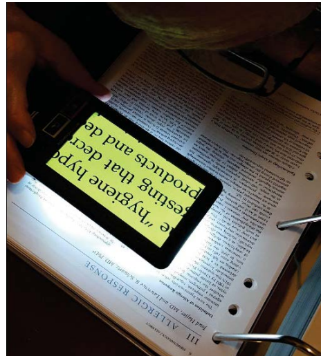
Figure 2. An electronic magnifier has a larger viewing area and the image can be manipulated to enhance contrast
